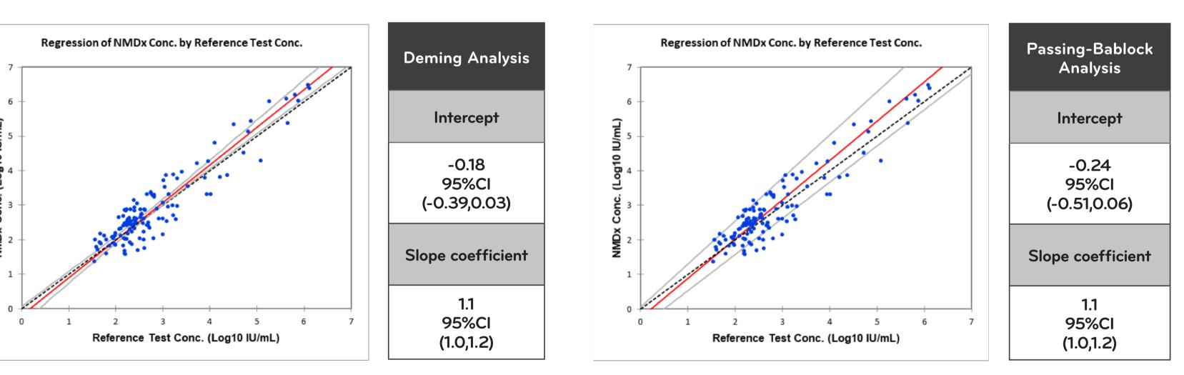
Clinical Quantitative Correlation of the NeuMoDx CMV Test. The NeuMoDx CMV Test demonstrated excellent quantitative correlation with an overall bias of either -0.18 Log10 IU/mL or -0.24 Log10 IU/mL for this quantitative study using either Deming linear regression analysis or Passing-Bablock analysis respectively.
