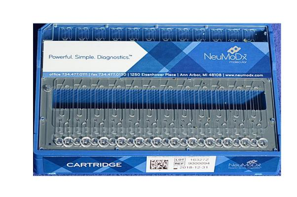
Patented microfluidic cartridges capable of performing independent sample processing and real-time PCR.
